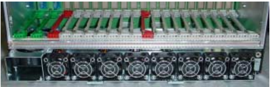
Figure 3-3. Fan Tray (partially withdrawn)
