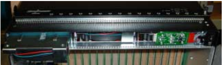
Figure 3-5. Cooling Blowers (one partially withdrawn)
